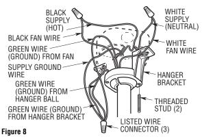
12. Securely connect the fan motor white wire to the supply white (neutral) wire using wire connector supplied (Figure 8). Securely connect the fan motor black wire to the supply black (hot) wire using wire connector supplied (Figure 8). After connections have been made, turn leads upward and carefully push the leads into the outlet box, with the wires spread apart and the white and green leads on one side of the outlet box and the black leads on the other side of the outlet box.
